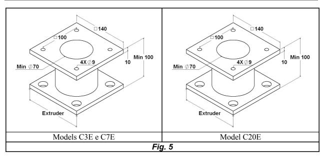
We recommend a very robust construction. In fact, it must withstand large forces and torque as well as strong vibrations. Should a material outlet for purging/cleaning purposes or closing valve are required, these cane be built on this flange. In case of any doubt or further information, please contact **IBE** or any of its representatives or distributors.
