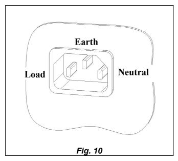
In order to avoid sporadic malfunctions of the microprocessor control, it is important to deliver a "clean" power supply to the **CONTGRAV**. A separate supply from a low impedance point should be installed.
