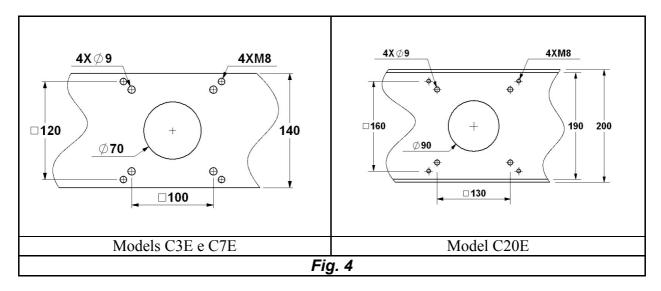
This structure should be assembled over a flange built by the installer, and has to adapt to the extruder on one side, and on the other to the **CONTGRAV** (see figure 5).
